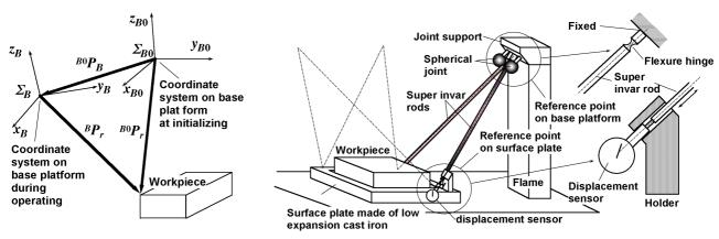
Fig.6 Two coordinate systems at initializing and during operating
