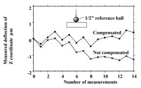
Fig.13 Variation of the measured coordinate during measurements
