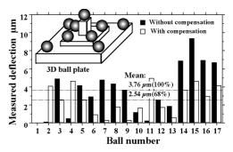
**Fig.12** Measured deflection of distances between the balls of 3D ball plate
