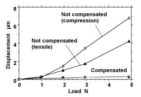
Fig.10 Differences of measured displacements between scale unit and laser interferometer
