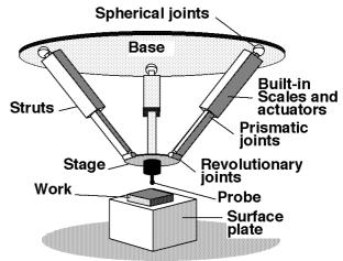
**Figure 1.** Proppsed CMM based on parallel mechanism
