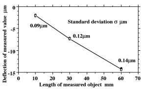
**Figure 5.** Deflection and standard deviation of measured data in Z direction before calibration
