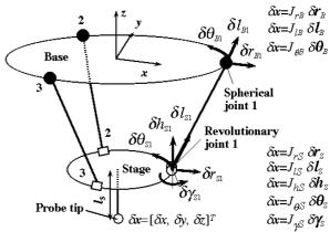
Figure 7. Motion errors of joints and probe tip
