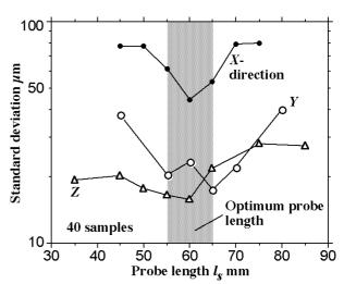
**Figure 10.** Influence of measuring point location on dispersion of measured value
