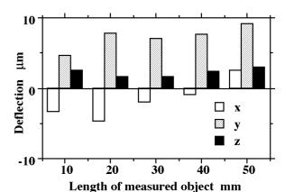
**Figure 6.** Deflection of measured data in XYZ directions after simple calibration
