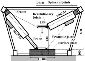
Figure 2. Scheme of experimental CMM
